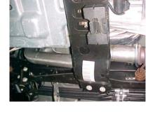
INSTALL PIPE #J ONTO PIPE #J. USE CLAMP #H TO SECURE PIPES TOGETHER. DO NOT TIGHTEN.
