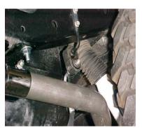
INSTALL THE OVERAXLE TAILPIPE #B INTO THE MUFFLER 1 ½" TO 2". SECURE TO THE MUFFLER USING CLAMP #D. DO NOT TIGHTEN. INSERT WELDED HANGERS INTO RUBBER GROMMETS. NOTE, SHORT END OF OVER AXLE PIPE INSERTS INTO MUFFLER.
