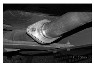
UNBOLT THE 2 BOLT FLANGE LOCATED BEHIND THE CATALITIC CONVERTER. SAVE STOCK NUTS AND BOLTS. YOU WILL REUSE THEM. NOW CUT OFF YOUR STOCK TAILPIPE JUST BEHIND THE MUFFLER AND REMOVE. LEAVE ALL RUBBER GROMMETS ON THE HANGER. USE WD-40 TO AID IN REMOVAL OF EXHAUST AND HANGERS.
