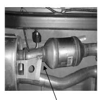
CUT BRACKET AT THIS POINT. THEN CUT 3/4" IN FRONT ON THE MUFFLER ON PASS. SIDE
