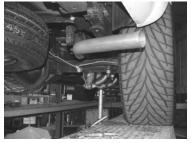
INTSALL THE PASSENGER OVERAXLE TAIL PIPE #C INTO MUFFLER OUTLET. SECURE WITH CLAMP #G.
