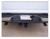
**8.** Install stainless steel tips #G. Clamp down. When you have everything in place, firmly tighten all bolts and clamps down securely. Use zip tie to secure brake/fuel lines away for exhaust. Use stainless steel cleaner and a Scotch Brite pad weekly to prevent tip from discoloration.
