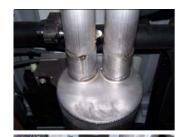
**6.** Install passenger tailpipe #E onto muffler 1½"-2" secure using clamp #I. DO NOT TIGHTEN. Insert welded hanger into rubber grommet.
