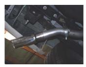
**7.** Install driver exit pipe #F onto tailpipe and secure with clamp #I. DO NOT TIGHTEN. Next, install passenger exit pipe #G and secure with clamp #I. DO NOT TIGHTEN.
