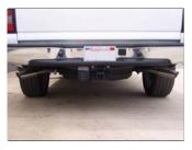
8. Install stainless steel tips #H. Clamp down. When you have everything in place, firmly tighten all bolts and clamps down securely. Use zip ties to secure brake/fuel lines away from exhaust. Use stainless steel cleaner and a Scotch Brite pad weekly to prevent tip from discoloration.
