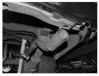
INSTALL EXIT PIPES # H
