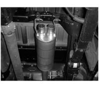
INSTALL MUFFLER #B ONTO HEADPIPE 1-1/2" TO 2" USING CLAMP #J. INSERT WELDED HANGERS INTO RUBBER GROMMET. MAKE SURE OUTLETS ARE LEVEL. USE A JACKSTAND TO SUPPORT MUFFLER. DO NOT TIGHTEN.
