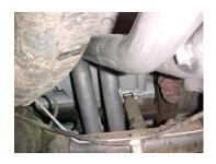
Install passenger side over axle tailpipe # C into muffler and attach using clamp # H. Use bolt kit # I to attach the tailpipes together. Insert hanger into rubber grommet. Do not tighten. YOU MAY NEED TO LOOSEN YOUR SPARE TIRE & PUSH TOWARDS DRIVER SIDE & RE-TIGHTEN.
