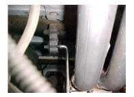
Install the driver side over axle tailpipe # D into the muffler. Use clamp # F to secure tailpipe to muffler. Do not tighten
