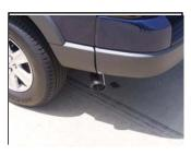
**6.** Install stainless steel tip #E. Clamp down. When you have everything in place, firmly tighten all bolts and clamps down securely. Use stainless steel cleaner and a Scotch Brite pad weekly to prevent tip from discoloration.
