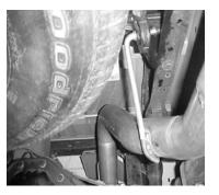
INSTALL OVERAXLE TAILPIPE #B AND CONNECT TO THE MUFFLER USING CLAMP # E. INSERT WELDED HANGERS INTO RUBBER GROMMETS.
