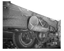
NEXT CONNECT THE TURN OUT PIPE #C TO THE OVERAXLE PIPE USING CLAMP #E. DO NOT TIGHTEN.
