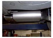
6. Install driver side muffler assembly #A. Insert welded hangers into rubber grommets. Use clamp #C to secure pipes together. Do not tighten.
