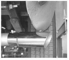
**INSTALL THE** STAINLESS STEEL TIP. NOW GO BACK AND TIGHTEN ALL CLAMPS, HANGERS, BOLTS AND FLANGE. TO CLEAN TIP USE ANY STAINLESS OR **ALUMINUM CLEANER** WITH A SCOTCH BRITE PAD.
