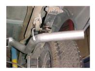
Install the exit pipe #D on to the tailpipe. Insert welded hanger into rubber grommet. Secure together with clamp #G. Do not tighten. Roll the exitpipe until it is at the correct angle for your truck.
