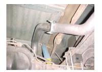
Install the over axle tailpipe #C into the muffler 1-1/2" to 2". Secure to the muffler using clamp #G. Do not tighten. Insert welded hanger into rubber grommet.
