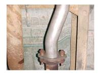
Install head pipe #A into flange #F. Bolt the flange and headpipe to the stock flange. Do not tighten.
