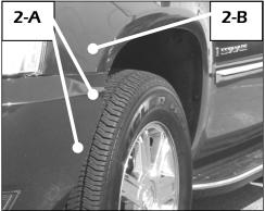
Remove the 7mm bolts and plastic fasteners attaching the inner plastic wheel wells to the bumper cover [2-A].
