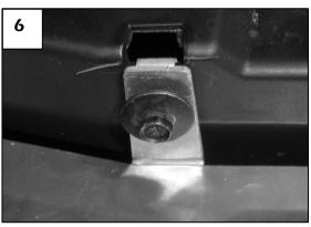
Test fit the grille into the opening. Trim additional material at cut edges (if needed). Remove grille. Install the top plate to the grille using the nylon lock nuts.
