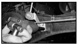
80. Working on the driver side, remove the emergency brake cable bracket from the bottom of the frame rail. Save the hardware.
