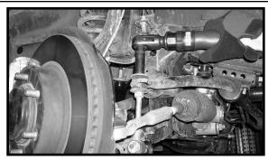
5. Working on the driver side, remove the sway bar from the OE location and save the hardware for later re-installation. Repeat procedure on passenger side. Set the sway bar a side for later re-installation.
