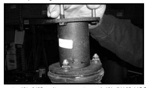
58. Locate (6) 3/8" unitorque nuts and (6) 5/16" USS flat washers from hardware bag 55900NB1. Working on the driver side, install the driver side strut back into the upper location and secure using the new 3/8" hardware. Make sure to add loctite and torque to 38 ft lbs. Repeat procedure on passenger side.
