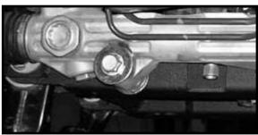
50. Locate (1) 9/16" x 2 1/2" bolt and (2) 1/2" USS flat washers from hardware bag 55900NB1. Also, locate (2) S10140 (9/16" fender washers) from hardware bag 55906NB2. Install the rack and pinion to the newly installed center rack and pinion bracket using the new 9/16" x 2 1/2" bolts, hardware and 9/16" fender washers. Special note: The fender washcenter rack and pinion bracket. Do not tighten at this of the rack and pinion downward.
