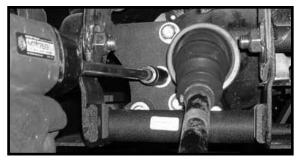
39. Move back to the new 1/2" hardware that connects the new driver and passenger side differential drop brackets to the newly installed one piece sub frame and add some loc-
