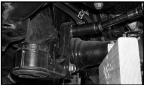
27. Using a tie down strap, carefully tie the front differential up and out of the way so that the hydraulic floor jacks can be removed and the one piece sub frame can be installed.
