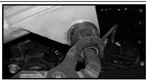
44. Locate (2) new MO3354 poly bushings and (1) S10075 sleeve from hardware bag 55900NB2. Working on the center of the rack and pinion, install the new bushings and sleeve into the rack and pinion. Special note: Make sure to use a lithium or moly base grease prior to inserting the new bushings and sleeve into the rack and pinion. This will increase the life of the bushings as well as prevent squeaking.
