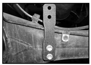
(2) 5/16" unitorque nuts from hardware bag 55900NB1 tite and torque to 16 ft lbs.
