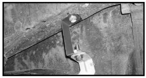
87. Locate the new rear brake proportioning valve bracket and the OE hardware. Install the new rear brake proportion-ware bag 55900NB2 and install them into the new ing valve bracket into the OE location and secure using the shocks. OE hardware. Make sure to use loctite and torque to 12 ft lbs.
