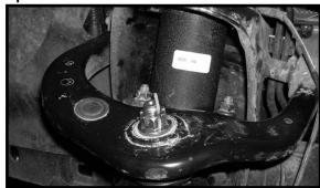
62. Working on the driver side, move back to the hardware attaching the upper control arm into the OE location and add some loctite and torque to 85 ft lbs. Repeat procedure on the passenger side.
