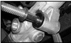
43. Carefully remove the bushing from the center of the rack and pinion and discard.
