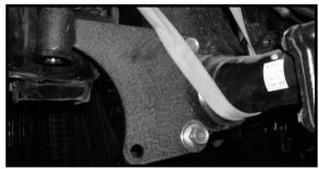
32. Locate the new one piece lower sub frame, (2) 3/4" x 4 1/2" bolts, (2) 3/4" x 5 1/2" bolts, (4) 3/4" unitorque nuts and (8) 3/4" flat washers from hardware bag 55900NB1. Install the new one piece sub frame to the front and rear lower control arm mounting points and secure using the new 3/4" bolts 28. Locate (1) new driver side differential drop bracket, (2) and hardware. Special Note: The new 3/4" x 5 1/2" bolt is
