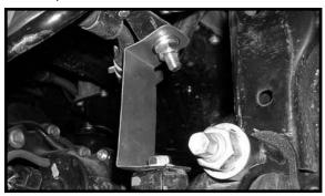
Working on the driver side, install the control arm back into the OE location. Secure using the OE hardware. Do not tighten at this point. Repeat procedure on the passenger new castle nut and the new upper ball joint are lined up and side.
