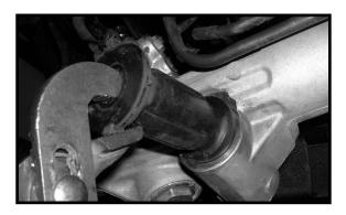
42. Locate (2) MO2382 poly bushings and (1) S10076 sleeve from hardware bag 55900NB2. Working on the driver side of the rack and pinion, install the new bushings and sleeve into the rack and pinion. Special note: Make sure to use a lithium or moly base grease prior to inserting the new bushings and sleeve into the rack and pinion. This will increase the life of the bushings as well as prevent squeaking.
