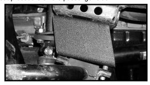
67. Locate the sway bar end link hardware. Working on the driver side, install the sway bar to the sway bar end link position and secure using the stock hardware. Make sure to use loctite and torque to 18 ft lbs. Repeat procedure on the passenger side.
