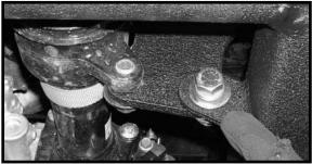
34. Locate the TOYRACK-02. Also, locate (2) 1/2" x 1 1/2" bolts, (4) 7/16" USS flat washers and (2) 1/2" unitorque nuts from hardware bag 55900NB1. Install the TOYRACK-02 to the rear portion of the newly installed one piece sub frame tite and torque to 85 ft. lbs. and secure using the new 1/2" hardware. Special note: make sure to install the bracket with the weld on the threaded spud is towards the ground. Do not tighten at this point.
