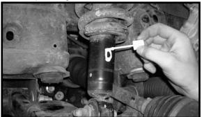
Working on the driver side, remove the (3) upper nuts that hold the strut assembly into the upper pocket. Save the hardware for later re-installation. Special note: DO NOT remove the upper center nut that holds the shock to the bearing plate. If the nut is removed, a coil spring compressor is going to be needed to put the strut assembly back ion to the sway bar mount. Repeat procedure on the pastogether. Repeat procedure on passenger side.
