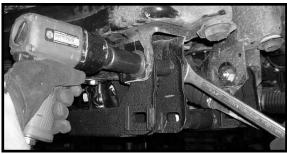
38. Move back to the stock hardware that connects the new driver and passenger side differential drop brackets to the front cross member and differential and add some loctite and torque all stock bolts to 85 ft. lbs.
