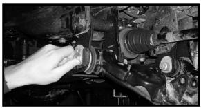
41. Carefully remove the bushing from the driver side of the rack and pinion and discard.
