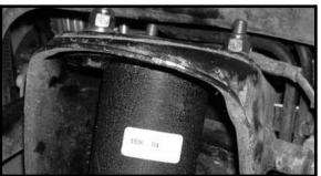
bag 55906NB2. Locate (1) 5/16" x 1" bolt, (2) 1/4" USS flat the driver side, secure the strut to the lower control arm washers and (1) 5/16" unitorque nut from hardware bag∎using the OE hardware. Make sure to use loctite and torque
