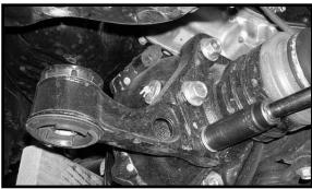
26. Working on the passenger side, remove the hardware that connect the differential drop bracket to the differential drop bracket may be discarded.
