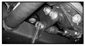
arm into the newly installed one piece sub frame and secure using the stock cam bolts. Center the stock cam bolt and torque 120 ft lbs. Repeat procedure on the passenger side.
