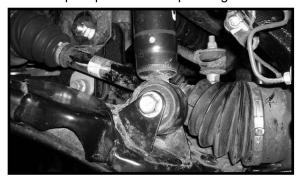
60. Locate the (2) bags that have the new ball joint spacers in them. Follow the instruction from Toyota on how to install the new dust boot cover on the new ball joints.
