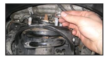
10. Working on the driver side, remove the lower mounting hardware that attaches the strut to the lower control arm. Save the hardware. Carefully lower down on the hydraulic floor jack allowing removal of the strut easier. Remove the strut and set aside. Repeat procedure on the passenger side.
