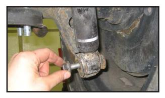
24. Working on the driver side, remove the u-bolts from the OE location. The u-bolts and hardware may be discarded. Place the lower u-bolt plate aside. Repeat procedure on the passenger side.
