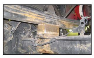
27. Locate (4) 9/16" x 2 9/16" x 9 5/8" square u-bolts. Locate (8) 9/16" u-bolt high nuts and (8) u-bolt washers from hardware bag 916NW. Also, locate the lower u-bolt plates. Working on the driver side, install the new u-bolts into the stock location and secure using the new 9/16" high nuts and washers. Special note: If need be, cut off the excess threads off each leg of the newly installed u-bolts. Torque to 120 ft lbs. Repeat procedure on passenger side.
