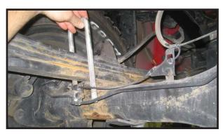
25. Carefully lower down on both hydraulic floor jacks at the same time allowing enough room for the rear blocks to be installed. Special note: Take special care not to over extend any brake lines and/or hoses.
