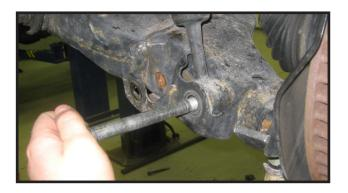
11. Carefully remove the struts from the vehicle.
