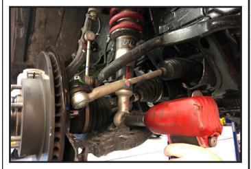
14. Locate and remove the 2 bolts that attach the lower control arm ball joint piece to the steering knuckle.
