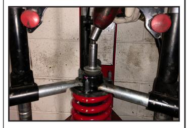
24. Remove the strut assembly from the strut compressor and take it back over to the vehicle. Locate part # 52907-01 and place it over the three studs.
