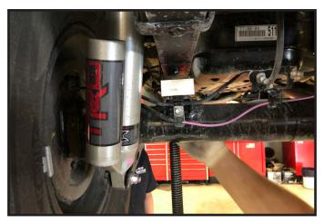
40. Locate the new rear u-bolts along with the new nuts and washers. Install the u-bolts and torque them to 150 ft lbs.
