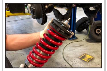
25. locate part # M10NLN and Install the strut back into the original location and use new nuts to loosely hold the strut in place.
