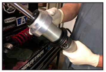
19. Remove the shock absorber from the strut assembly out 21. Re-install the plastic dust boot and metal washer of the bottom of the coil spring. Remove the metal washer and plastic dust boot. Save for re-installation
