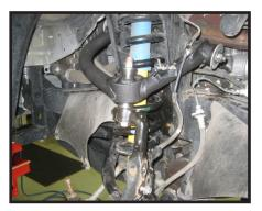
11. Working on the driver side, locate (1) 1/4" nylock nut and (1) 1/4" USS flat washer. Attach the OE ABS brake wire bracket to the new upper control arm. Repeat on passenger side.
