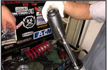
18. Carefully compress the strut until the upper hardware and save over the body of the shock. **Make sure to install the new** for re-assembly. **Spacer so that the "coil shelf" is facing upwards.**
