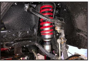
26. Raise the lower control arm back up until you can install the OE lower mounting bolt and hardware. Leave this loose for now.
