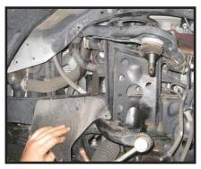
5. Using a pair of large channel locks or similar type tool, Bend the pinch welded lip of the inner fender just enough that the upper control arm bolt will be able to be completely removed. Remove bolt and save. Repeat on passenger side.
