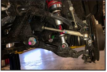
27. Raise the lower control arm up even more until you can re-install the 2 lower ball joint bracket bolts to the steering knuckle. Torque to 160 ft lbs.
