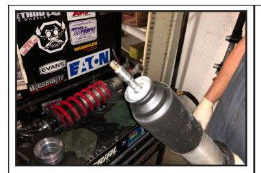
22. Re-install the shock absorber into the strut assembly an make sure to line up your reference marks made on step #8.
