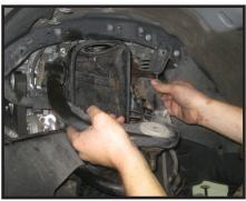
7. Locate the new upper control arms. Locate (8) poly bushings and (4) S10248 sleeves from hardware bag 50930PL, Install the new bushings and sleeves into the new upper control arms. **Special note: Make sure to use a fair amount of lithium or moly base grease before installing the new bushings and sleeves into the control arms. This will increase the life of the bushing as well as help prevent squeaking.**
