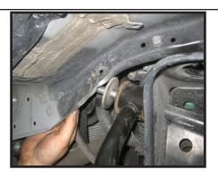
4. Working on the driver side, Remove plastic clips holding rubber spray gaurds to the inner fender. Only remove enough to get to the upper control arm bolt. Repeat on Passenger side.
