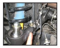
12. Working on the driver side, remove 2 of the upper strut mounting nuts, and leave 1 of them loosely threaded on to hold strut into the vehicle.
