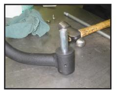
8. Locate the new sert fittings from hardware bag 50930PL. Install the new sert fittings into the new upper access when using a grease gun.
