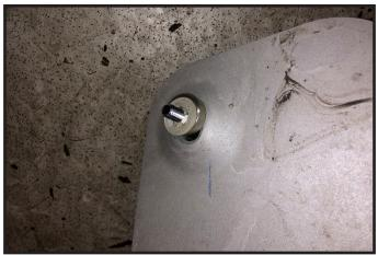
33. Once the required spacer sleeves and hardware have been installed, lift the skid plate back into place and secure all 6 mounting bolts to their OE locations. Torque to 20 ft lbs.
