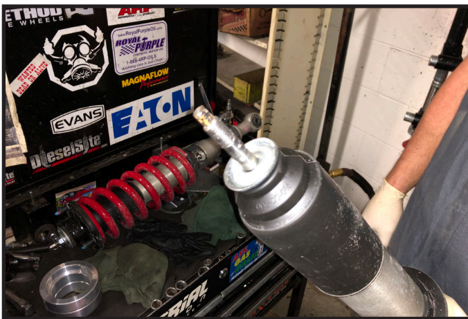
13. Re-install the shock absorber into the strut assembly and make sure to line up your reference marks made on step #8.
