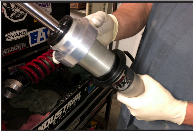
12. Re-install the plastic dust boot and metal washer
