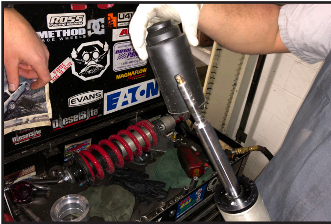
12. Re-install the plastic dust boot and metal washer
