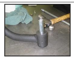
7. Locate the new sert fittings from hardware bag 50930PL. Install the new sert fittings into the new upper control arms. Special note: Make sure not to over tighten and also make sure that the sert fitting is facing towards the outside of the vehicle. This will make for easier access when using a grease gun.
