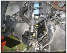
10. Working on the driver side, locate (1) 1/4" nylock nut and (1) 1/4" USS flat washer. Attach the OE ABS brake wire bracket to the new upper control arm. Repeat on passenger side.
