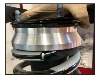
11. Making sure to line up your reference marks from step #7, Carefully compress the strut assembly back together and re-install the OE nut. Torque to **30 ft lbs.**
