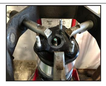
12. Re-install the strut assembly into the vehcle and hold in place using the 3 OE nuts. **Do not tighten at this point.**
