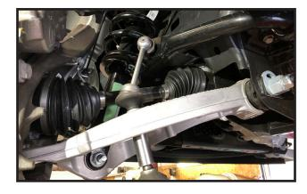
3. Remove the lower strut mounting hardware at the lower control arm and save the hardware.
