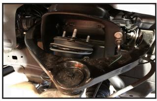
7. Place the strut assembly into a wall mounted strut compressor, and make a reference mark on the top hat so that it can be re-installed in the same direction. Special Note: If you do not have a wall mounted strut compressor, you will need to take the struts and new strut spacers to a certified technician to perform these steps.
