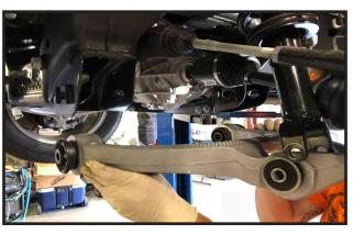
6. Move to the upper strut mounting hardware and remove the 3 nuts. Carefully lower the strut assembly out of the vehicle.
