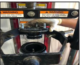
10. Install the new aluminum strut spacer on top of the coil spring. The order of pieces once in stalled are as follows: from the top down: OE top hat, OE rubber isolator, New factory strut spacer, OE dust shield, OE plastic spring lock.
