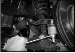
5. Now return to the upper ball joint and outer tie rod and carefully break the taper and remove them both from the steering knuckle. Repeat on passenger side. Special Note: Take special care not to damage the ball joint and tie rod end rubber boots.
