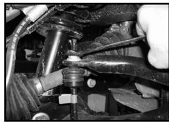
7. Working on the driver side, remove the nut and bolt holding the strut assembly to the lower control arm. Repeat on passenger side.
