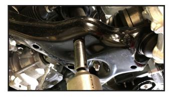
Remove the driver and passenger side lower conrol arm cam bolt nuts. Save hardware.
