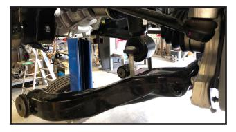
Working on the top strut mounts. Remove the three nuts that holds the srut, and remove the strut. Careful, the strut will fall if its not held when last nut is removed. Repeat on passenger side.
