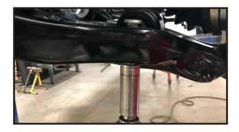
13. On driver and passenger, Raise the lower control arm 16. Working on the top strut mounts. Tighten the three nuts
