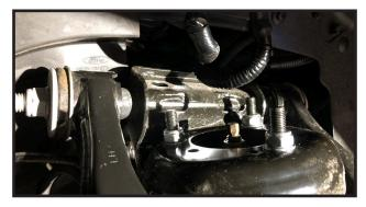
up to the lower strut mount. Locate the OE lower studs and to 30 ft-lbs nuts. Install them into the strut and lower control arm. Leave loose
