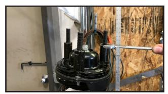
11. Locate the strut spacers part # M09151-BK-01. Slide spacer over the stud extenders, so its seated flat on the top hat.
