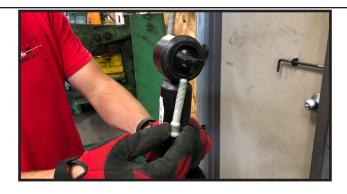
10. Locate locktite from hardware bag. Put locktite on the three studs on the strut top hat.
