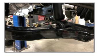
14. Locate OE lower control arm cam bolt hardware. Using a jack, Raise lower control arms into frame mounts. Install Carefully lower the vehicle back down to the ground and front and rear cam bolts and nuts into lower control arm remove the jacks. mounts. Leave loose.
