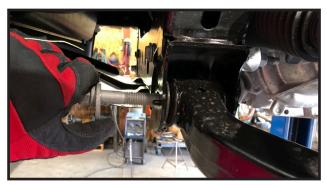
5. Lower the lower control arm out of the mounting pocket on the driver and passenger side.
