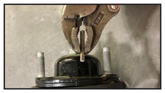
Using a hammer and a vice. Remove the two studs on the lower strut mount. Thread the nut on the stud to prevent damage to the stud. Save Hardware.
