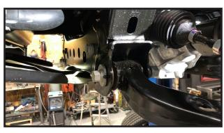
15. Tighten the lower strut studs tell there pulled in all the way in flush. Back the nut off one turn, Then Tighten to 90f t lbs.
