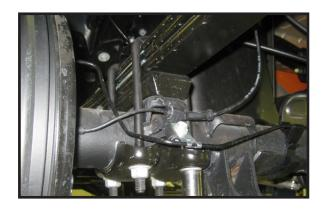
43. Carefully lower down both hydraulic floor jacks at the Repeat procedure on passenger side. same time approximately 3". Special note: Take special care not to over extend any brake lines and/or hoses. Working on the driver side, remove and discard the stock rear block. Repeat procedure on the passenger side.
