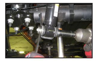
42. Working on the driver side, remove the u-bolts from the OE location and discard the u-bolts and hardware. Set the upper and lower u-bolt plates aside for later re-installation. Repeat procedure on passenger side.
