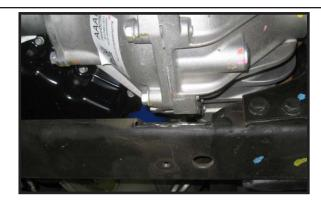
12. Working on the driver side, remove the ABS line from the bracket on the top of the upper control arm pocket. Now disconnect the ABS lines from each other at the quick disconnect. Special note: Take special care not to damage ABS line during removal. Repeat procedure on the passenger side.
