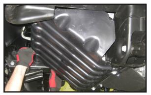
Working on the driver side, center and torque the OE cam bolts to **95 ft lbs.** Repeat procedure on the passenger side.
