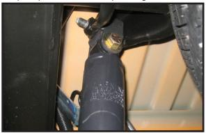
49. Locate the new zip tie in hardware bag 14059PL. Working on the driver side, zip tie the ABS line to the OE bump stop bracket. Repeat procedure on the passenger side.
