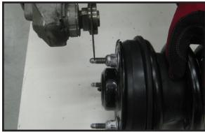
25. Locate the new upper strut spacers. Install the new spacers to the OE struts and secure using the OE hardware. Make sure to use loctite.
