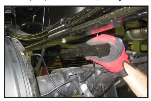
side, install the new 3" lifted block into the stock location, point. Repeat procedure on the passenger side.
