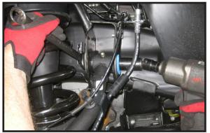
35. Working on the driver side, grease the upper control arm bushings and ball joint. Repeat procedure on the passenger side. Special note to the customer: Make sure to have the upper control arm bushings and ball joints greased each time you have the oil changed.
