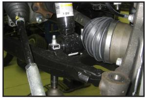
17. Working on the driver side, remove the upper clips off the upper strut studs. Remove the nuts holding the strut into the 15. Working on the driver side, remove the outer tie rod from upper location and save. Remove the strut from the vehicle the OE knuckle. Save the hardware. Special note: Using and remove and discard the lower attaching clips. Set the
