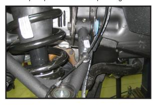
30. Working on the driver side, install the outer tie rod to the OE knuckle using the OE hardware. Make sure to use loctite and torque to 95 ft lbs. Repeat procedure on the passenger side.
