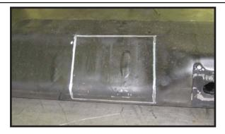
10. Using a die grinder, carefully notch out the OE cross member following the lines that were scribed earlier.
