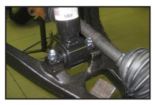
28. Remove the cotter pins and castle nuts from the newly installed control arms. Working on the driver side, install the newly installed upper control arm to the OE knuckle and secure using the new castle nut. Make sure to use loctite and torque to 40 ft lbs. Now install the new cotter pin. 29. Locate (2) 6 mm flat washers and (2) 6 mm unitorque can be installed. Repeat procedure on the passenger side. frame rail. Repeat procedure on the passenger side.
