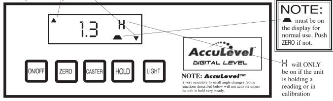
**NOTE:** This Ver. 5 Acculevel<sup>™</sup> has 2 modes of operation. 1) In Normal angle measurement mode the display is steady. 2) In Caster Mode the display flashes (and will not measure absolute angles). Push CASTER button to exit Caster mode and go back to Normal angle measurement.
