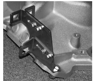
Figure 2 - Manifolds 52000/52001, 52006/52007, 52008/52009, and 53000/53001 are designed to accept the stock style spread bore carburetor. To use a square bore carb, you must utilize the supplied carb adapter plate and gasket or air leakage will occur at the base of the carburetor.
