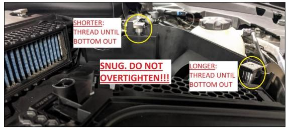
3) Place Dinan engine cover into place. You should hear an audible CLINK, CLINK, CLINK. This lid should self-align with the magnets. Small adjustments can be made if needed.
