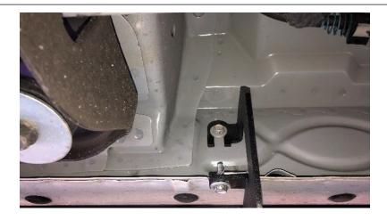
**Step 8:** There will be  $\frac{1}{2}$ " of adjustment in the (x3) mounting bracket. Adjust to desired position and tighten to (20 ft,/lbs).
