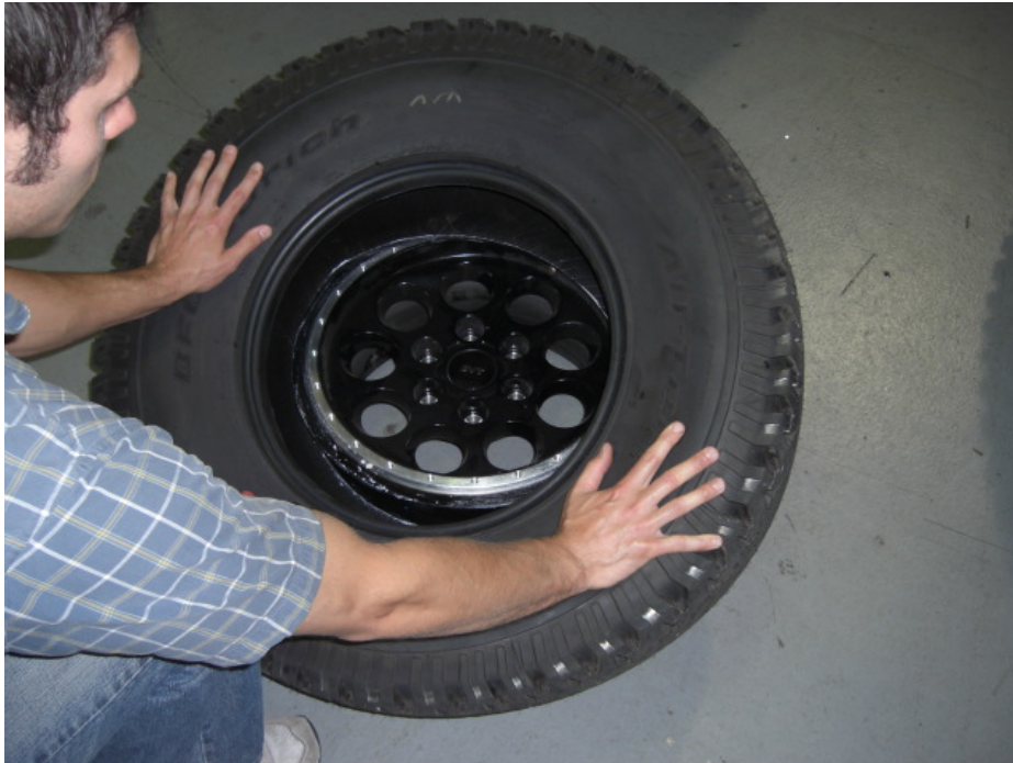
Pic 2.1 – Force the inner tire bead over outer wheel flange.
