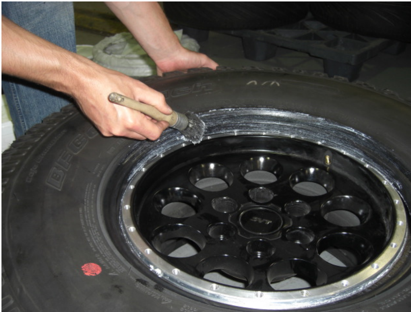
Pic 4.1 – Apply a liberal amount of tire soap to the entire bead.
