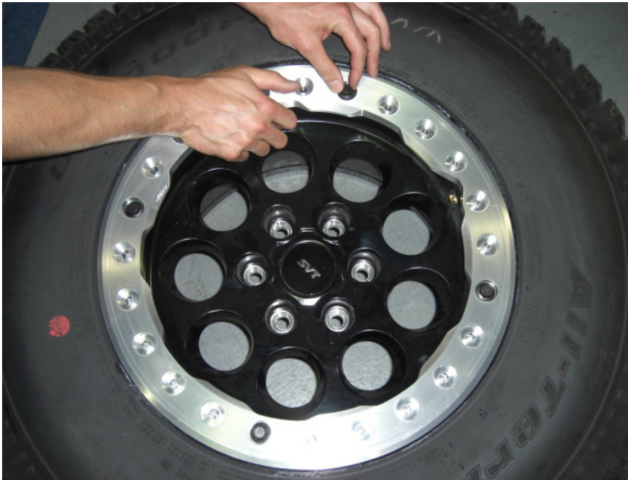
Pic 5.1 – Hand thread 4 bolts at the corners.
