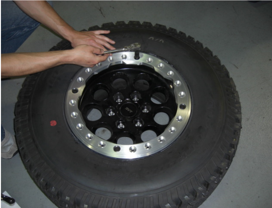
Pic 5.2 – Tighten each bolt at least one turn with a socket wrench.
