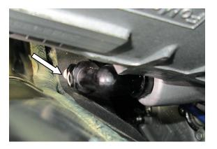
**STEP 14:** Feed the new hydraulic clutch line down the elbow on the transmission housing, lubricate the O-ring and gently push the new hydraulic clutch line end into the clutch cylinder housing until it locks into the retaining clip
