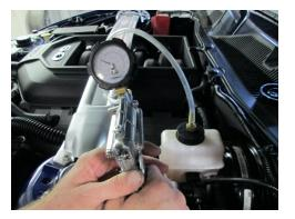
**STEP 21:** Holding the rubber stopper in place, operate the vacuum pump to 15-20 inches of vacuum. Hold the vacuum for 1 minute, then quickly relieve the vacuum. Remove the special tools.
