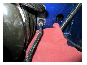
**STEP 5:** Using a small pick, gently pull the hydraulic hose retaining clip outboard to release the hose.
