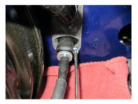
STEP 6: Gently pull the hydraulic hose out of the clutch cylinder housing.
