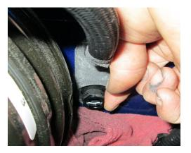
**STEP 12:** Lubricate the O-ring and gently push the new hydraulic clutch line end into the clutch cylinder housing until it locks into the retaining clip.
