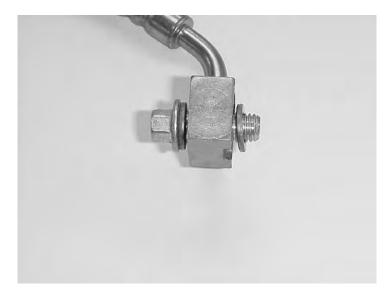
**STEP 30:** Secure parking brake cables to calipers as shown.
