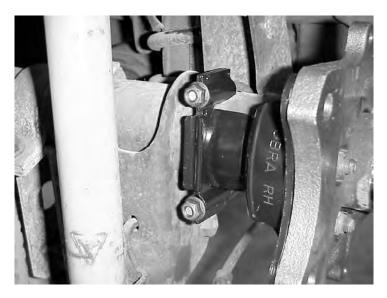
**STEP 26:** Install new rear rotors (Item 5) on the axle using a lug nut to temporarily hold the rotor in place.
