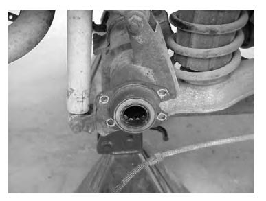
**STEP 11:** Reusing the backing plate bolts, install the caliper to axle adapters (item 1 and 2). Torque bolts to 45-50 ft./lbs. Axle adapters are marked LH and RH. The RH is shown below.
