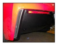
3) On the outside ends of each side of the bumper fascia there are small, plastic, vertical grates that must be removed. These are held in place by small clips. Use a small screwdriver to carefully pop these out. At the bottom, where the red and black panels touch, they clip together. Use a small flat blade screwdriver to carefully separate them.
