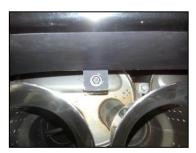
In the cavity just above the exhaust tips, there are two last hex bolts that need to be removed. At this point the panel is ready to be removed. We recommend that you have a helper for this part. The panel is secured along the top edge with clips. Grasp the panel at one end through the vertical slot and carefully pull it out. This will take a little muscle and finesse but it should pop right off. Once it's off, place it in a safe area out of the way.
