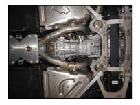
Just forward of the rear sub-frame and axles you will find a clamp connection on each of the pipes. Loosen the nut on each of these clamps. Also, up at the top on each of the pipes that run over the axle, and the outer exhaust tip at the rear of the mufflers, there is an electrical butterfly actuator. Disconnect the electrical connectors at each of these actuators.
