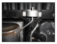
Above the outer edge of each muffler there is a hanger bracket bolted to the frame that supports the muffler. Remove the bolts that secure one side. Once it's off you should be able to wiggle the muffler assembly loose from the front connection and then out from over the axle. Repeat for the other side. Slip the hanger brackets off the original mufflers and slip them on to the new Flowmaster mufflers.
