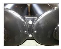
12) Once both mufflers are in place and supported, there are small brackets at the rear that will connect them together. Use the two supplied button head bolts, nuts and washers to secure the two mufflers together. Reconnect the electrical connectors to the actuators on the new mufflers.
