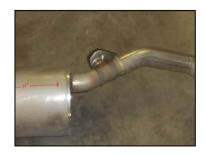
9) With the original mufflers out of the vehicle, remove the butterfly actuators that are mounted to the pipes just forward of the mufflers and at the outer tip. These are secured by three small hex head screws.
