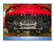
11) Once the actuators have been installed onto the muffler assemblies, the system can be reinstalled on the vehicle. Position one muffler at a time, up over the axle into the clamped connection. Re-use the original bolts to secure the rear hanger bracket up to the frame.
