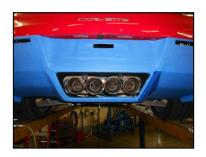
1) The entire lower rear bumper fascia (Blue portion in photo) must be removed. Because this is a painted body panel, you may want to consider covering it with masking tape for the disassembly/assembly process to prevent any scratches. Note: Do not turn the vehicle ignition on anytime during the removal/assembly process.
