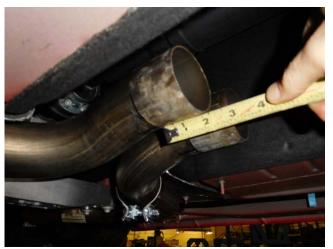
3) Begin the installation by placing a supplied 2-3/4" clamp onto each of the inlets of the Scavenger pipe #26522S. Then place the Scavenger pipe onto the back of the stock head pipes (the offset outlet pipe should be oriented to the passenger side). Level and center the assembly in the drive line tunnel and support with a stand. Scavenger pipe should slide over factory head pipe about 2". Tighten the two clamps enough to hold, but still allow for adjustment.
