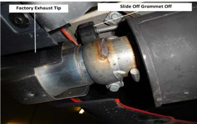
5) Once the factory system is out of the vehicle, use a 5/16" wrench to remove the three nuts securing the actuator to the mounts on the tailpipes. Remove the actuator and spring from the mount on each tailpipe.
