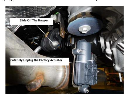
4) Slide the three hangers on each tailpipe out of the rubber mounts on the vehicle and unclip the grounding strap from the rear hanger on the right side of the vehicle. The stock system will come out as one large unit. Carefully lower the stands at the rear of the vehicle and with the help of an assistant slide the system back off of the head pipes and lower the system from the vehicle.
