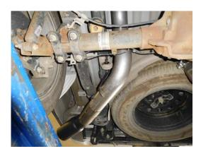
4) Install a provided clamp onto the muffler outlet. Then place tailpipe **#46197S** into position over the axle and into the muffler outlet while also connecting the hangers on the pipe to the rubber mounts on the vehicle. Tighten the band clamp enough to hold, but still allow for adjustment.
