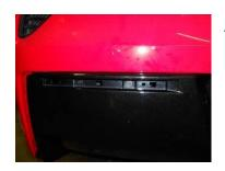
4) On each side of the bumper fascia there is a thin horizontal red reflector that must be removed. It is held in place with clips. Use a small flat blade screw driver to very carefully pop out these two reflectors. Once the reflectors are removed, you will see two hex bolts that secure the fascia to the bumper frame. Remove these two bolts along with two that are located under where the license plate was mounted.
