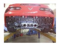
This is what things should look like now. Now you need to start working under the car so either put the car on a hoist, or put the rear of the car on jack stands or ramps. At the rear, between the two factory mufflers you will find that they are connected by small brackets that are secured with small hex bolts. Remove these so that the mufflers can be removed separately.
