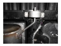
Above the outer edge of each muffler there is a hanger bracket bolted to the frame that supports the muffler. Remove the bolts that secure one side. Once it's off you should be able to wiggle the muffler assembly loose from the front connection and then out from over the axle. Repeat for the other side. Slip the hanger brackets off the original mufflers and slip them on to the new mufflers.
