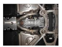
7) Just forward of the rear sub-frame and axles you will find a clamp connection on each of the pipes. Loosen the nut on each of these clamps. Up at the top on each of the pipes that run over the axle, there is an electrical butterfly actuator. Disconnect the electrical connectors.
