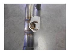
10) Using the three hex head screws removed in the step above install the butterfly actuators onto the valves in the new Flowmaster muffler assemblies. Tighten the three screws securely.
