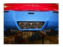
1) Before you begin, please understand that the installation of this system requires significant disassembly. The entire lower rear bumper fascia (Blue portion in photo) must be removed. Because this is a painted body panel, you may want to consider covering it with masking tape for the disassembly/assembly process to prevent any scratches. Note: Do not turn the vehicle ignition on anytime during the removal/assembly process
