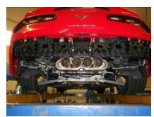
11) Once the actuators have been installed onto the muffler assemblies, the system can be reinstalled on the vehicle. Position one muffler at a time, up over the axle into the clamped connection. Re-use the original bolts to secure the rear hanger bracket up to the frame.
