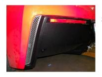
On outside ends of each side of the bumper fascia there are small, plastic vertical grates that must be removed. These are held in place by small clips. Use a small screwdriver to carefully pop these out. At the bottom, where the red and black panels touch, they clip together. Use a small flat blade screwdriver to carefully separate them.
