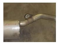
9) With the original mufflers out of the vehicle, remove the butterfly actuators that are mounted to the pipes just forward of the mufflers. These are secured by three small hex head screws.
