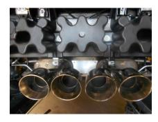
12) Once both mufflers are in place and supported, there are small brackets at the rear that will connect them together. Use the two supplied button head bolts, nuts and washers to secure the two mufflers together. Reconnect the electrical connectors to the actuators on the new mufflers.
