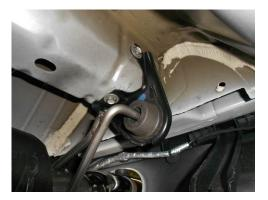
3) Using a 13mm wrench, unbolt the two hangers just behind the rear differential from the cross member. Now, with the help of an assistant, carefully lower the center stand and slide the exhaust system forward and out of the rear hanger mounts. Lower the system to the floor leaving the front hangers attached. Finally remove the two hanger mounts at the rear of the vehicle from the frame using a 13mm wrench. As you remove them, place them with the factory muffler from the corresponding side.
