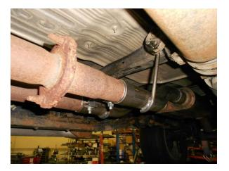
1) After removing any burrs, use a tape measure to measure back 3.00" from the pipe edge on each inlet pipe and make a mark. Place a supplied clamp onto each inlet pipe of muffler **8430013-420**. Place the muffler assembly up into position and slide onto the factory front pipes up to the line at 3.00", then connect the hangers on the muffler to the rubber mounts on the vehicle. Level the muffler and tighten the clamps securely.
