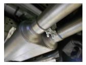
8) Install a provided 2½" clamp onto the right muffler outlet. Place the right side tailpipe **#86195S** into position over the axle and slip into the right side muffler outlet, while at the same time, connecting the hangers at the front and rear of the pipe to the rubber mounts on the vehicle. Tighten the clamp enough to hold, but still allow for adjustment.
