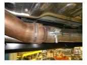
4) Trim inlet pipe **#26428S** according to the following measurements before placing onto the stock front pipe just behind the catalytic converter. Be sure to line up the notch in the pipe with the tab on the front pipe. Place the provided 3" clamp onto this connection and tighten enough to hold.
