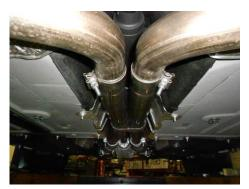
5) Begin the installation by placing a supplied 2-3/4" clamp onto each of the inlets of the Scavenger pipe **#26591S.** Then place the Scavenger pipe onto the back of the stock head pipes (the offset outlet pipe should be oriented to the passenger side). Level and center the assembly in the drive line tunnel and support with a stand. Tighten the two clamps enough to hold, but still allow for adjustment.
