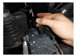
8) Reconnect the two electrical plugs removed in step 2 of the removal instructions back onto the tailpipe actuators now installed on the new Flowmaster tailpipes.
