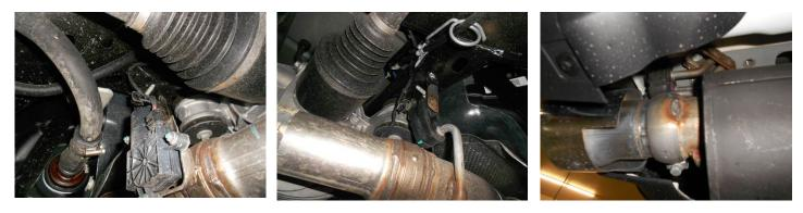
3) Once the factory system is out of the vehicle, use a 5/16" wrench to remove the three nuts securing the actuator to the mounts on the tailpipes. Remove the actuator and spring from the mount on each tailpipe.
