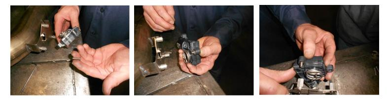
4) Be sure that the center arm of the actuator spring is between the bottom and top tabs of the mount, tighten all three bolts securely. Repeat the step on the other tailpipe assembly.
