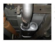
3) Place a provided 3½" clamp onto the outlet of the muffler, then place tailpipe #36057S into position over the axle and connect it to the muffler outlet. Connect the wire hanger at the front and rear of the tailpipe to the rubber mounts on the vehicle.
