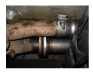
1) Install resonator assembly **#15129S** by first sliding a 2 1/2" clamp onto the left inlet pipe, then put the assembly up into place and align the flange connection on the right side and the slip joint on the left side. Reinstall the two nuts onto the flange. Tighten the clamp and flange nuts enough to hold, but still allow for adjustment.
