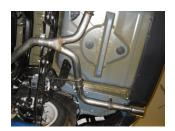
7) On the right side of the vehicle, place a supplied 2.25" onto the expanded end of exit pipe **#86019S** and slide onto the right outlet of the Y-pipe. Connect the hanger on the pipe to the rubber mount on the vehicle and tighten the clamp enough to hold, but still allow for adjustment.
