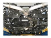
6) Place a supplied 2.50" clamp onto the inlet of Y-pipe assembly **#86016S**, place onto the back of the mid pipe and seat the two pipes fully together. Connect the two hangers on the y-pipe to the rubber mounts on the vehicle and tighten the clamp enough to hold, but still allow for adjustment.
