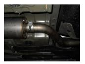
5) Place a supplied 2.50" clamp onto the muffler outlet, then place mid pipe **#86015S** into the muffler outlet and rotate into position. Support the back of the pipe with a stand and tighten the clamp enough to hold but still allow for adjustment.
