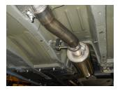
4) Place a supplied 2.50" clamp onto the inlet of muffler **12514310-Z** and fully seat onto the back of inlet pipe **#86014S**. Support the muffler with a stand and tighten the clamp enough to hold but still allow for adjustment.
