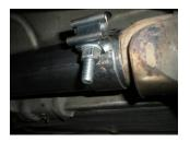
Place a provided 2.25" clamp onto the slip-fit of inlet pipe #TB566S then place onto the back of the catalytic converter. Tighten the clamp enough to hold, but still allow for adjustment.
