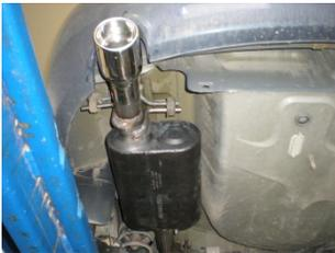
8) Place the **ST339** stainless tip onto the muffler outlet and adjust to the desired position. Tighten the clamp enough to hold, but still allow for adjustment.
