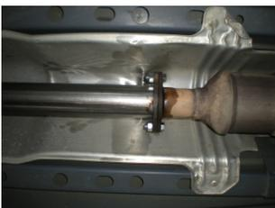
5) Place inlet pipe **#16768S** onto the back of the catalytic converter and then using the 3/8" nuts, bolts and washers provided, bolt the two flanges together and tighten securely. Connect the hanger at the back of the pipe to the rubber mount on the vehicle.
