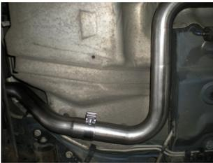
6) Place a provided clamp onto the expanded end of over-axle pipe **#16769S** and slide onto the back of the inlet pipe **#16768S**. Rotate the pipe up into its approximate position and connect the hanger on the pipe to the rubber mount on the vehicle. Tighten the clamp enough to hold, but still allow for adjustment.
