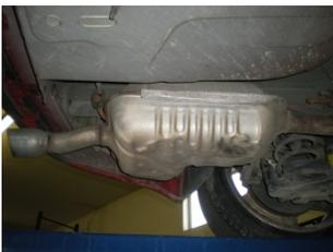
4) At the rear of the vehicle, remove the three hangers on the muffler and over-axle pipe assembly from the rubber mounts on the vehicle and lower the stock muffler from the vehicle.
