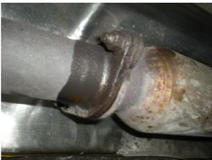
3) Remove the two nuts attaching the factory mid pipe to the rear of the catalytic converter. Once the flange is loose, remove the hanger at the rear of the pipe from the rubber mount on the vehicle and lower the pipe from the vehicle.
