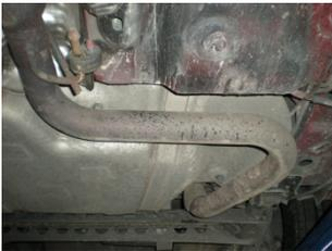
2) In order to remove the stock system from the vehicle, the system will need to be cut in half. Support the rear muffler with a stand, then using a hacksaw or sawzall, cut the pipe just before it passes over the rear axle.
