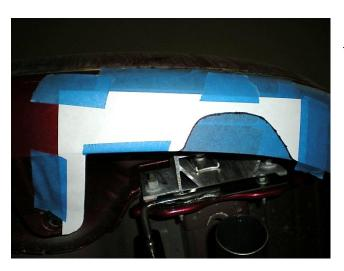
3) Use a marker and trace the cut-out template onto the masking tape. Remove the template after marking.
