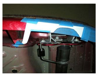
2) Use scissors to carefully cut out one of the provided paper templates and securely tape it to the bumper. Make sure to follow the lines on the body as well as the bumper mount to line up the template properly. There are two templates included, one for the R/S package bumper and one for the standard models.
