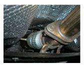
3) In front of the large center muffler, remove the two nuts at the flanged connection just behind the flex joint. Then remove the two bolts from the steel body brace behind the large muffler. Once unbolted, remove the hanger on this section from the rubber mount on the vehicle and lower from the vehicle and set aside. Save the gasket from between the two flanges for use with the Flowmaster system.
