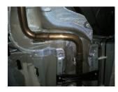
5) Place a supplied clamp onto the expanded end of pipe **#16738S** and slide onto the back of the resonator. Connect the hanger on the pipe to the rubber mount on the vehicle and tighten the clamp just enough to hold, but still allow for adjustment.
