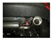
9) Place the wire hanger of clamp hanger **#440HA** into the rubber mount on the vehicle and then place the clamp over the muffler outlet. Place exit pipe **#16741S** into the muffler outlet and tighten the clamp enough to hold, but still allow for adjustment. Place the stainless tip **#ST339** onto the end of the exit pipe and adjust to the desired position. Tighten the clamp on the tip enough to hold, but still allow for adjustment.
