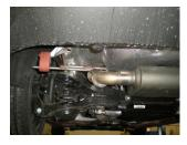
7) To install muffler inlet pipe **#16740S**, remove the two bolts that attach the drivers' side muffler hanger to the frame, turn the hanger 180 degrees so that it is pointing to the outside of the vehicle and reinstall. Place a supplied clamp onto the expanded end of pipe **#16740S**. Connect the hanger on the pipe to the rubber mount on the vehicle then slide onto the back of pipe **#16739S**. Tighten the clamp enough to hold, but still allow for adjustment.
