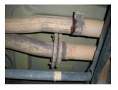
3) Separate the wire hangers in front and back of the muffler from their rubber mounts on the vehicle. Remove the two nuts from the flanged connection on the right inlet pipe using a 15mm wrench. Loosen the nut on the band clamp on the left inlet pipe. Slide the muffler assembly toward the rear of the vehicle and off of the left inlet pipe. Lower the muffler assembly from the vehicle.
