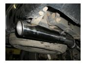
10) Place the ST396 stainless tips onto the ends of the tailpipes and adjust to the desired location. Tighten the nut on the clamp to secure the tip in place.
