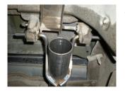
4) Connect the two hangers at the rear of inlet pipe **#16695S** to the rubber mounts on the vehicle and support the front of the pipe with a stand.
