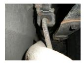
3) Separate the two wire hangers on the tailpipe from the rubber mounts on the vehicle. Remove the tailpipe and set aside.
