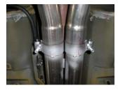
Place a 2<sup>1</sup>/<sub>4</sub>" clamp onto the slip-fit of over-axle pipe **#16679S** and slide onto the back 6) of the right Scavenger outlet and support with a stand. Repeat this step with the left over-axle pipe #16680S.
