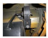
Install the OEM hanger bracket removed from the rear of the factory muffler onto the 7) rear hanger of muffler #852467-229. Place the muffler up into position and connect the muffler inlet to the over-axle pipe. Bolt the hanger bracket to the frame using the OEM hardware. Connect the hanger on the front of the muffler to the factory mount on the vehicle.
