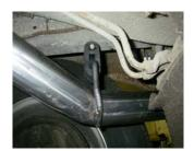
8) Place right tailpipe **#16703S** over the rear axle and so that the rear of the tailpipe exits between the quarter panel and the leaf spring. Place the hanger at the rear of the pipe into the rubber mount installed in step 3 above. Then slide the front of the tailpipe through hanger **#389HA**. Do the same for the left tailpipe **#16704S**.
